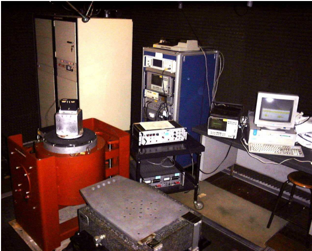
Fig. 17. USO mounted on the shaker during vibration test
